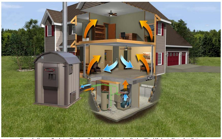
Figure 1: Concept Rendering Showing a Typical Installation of an Outdoor Wood Hydronic Heater Installation
